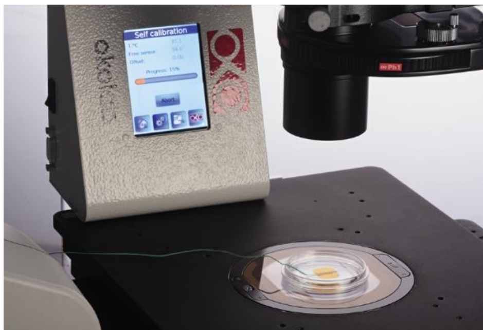
Figure 16 Example of a petri dish with Fine Gauge Thermocouple placed onto a Thermal Plate.
