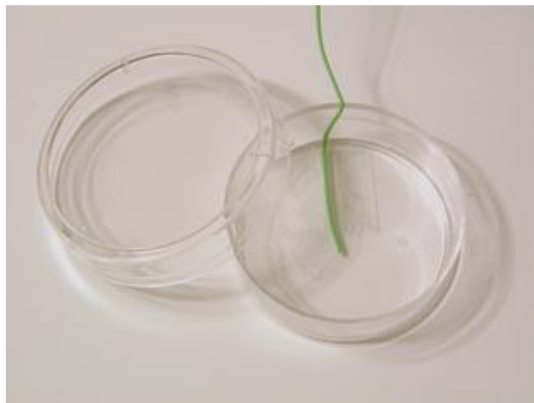
Figure 49. Free Sensor attached on the internal base of the Petri Dish
