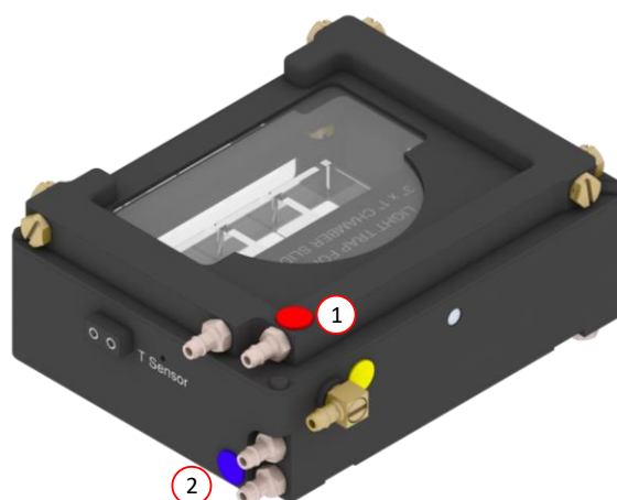
Figure 14. Connection with the thermostatic bath.
